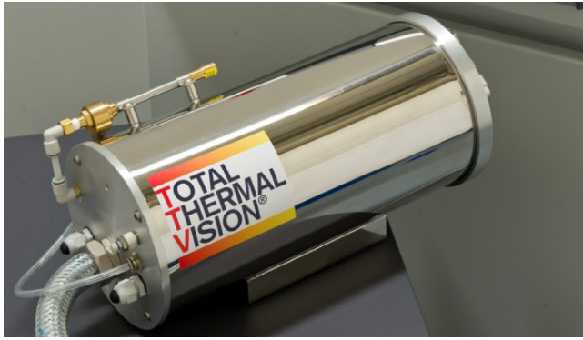
Figure 10 – Total Thermal Vision® from Baraldi can read and store the die skin temperature at each cycle of the machine by monitoring the entire die with an IR camera mounted in a protective stainless steel case.
