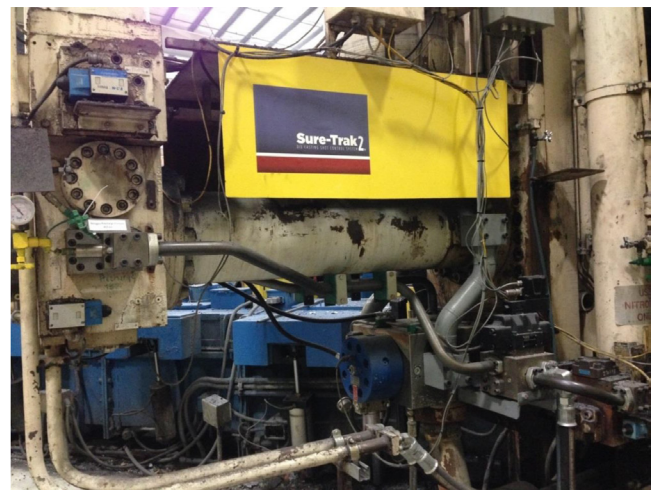
Figure 8 – View from the Helper side – 1 year of operation with no components replaced and no downtimes for Hydraulic Leaks on the Shot End.
