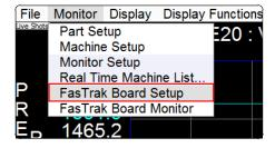
When the FasTrak Board Setup dialog appears, check the "Address" of the FasTrak2 board, pointed to on the picture below, and make sure it is the same as the actual address of the FasTrak2 board that you are trying to connect to.
